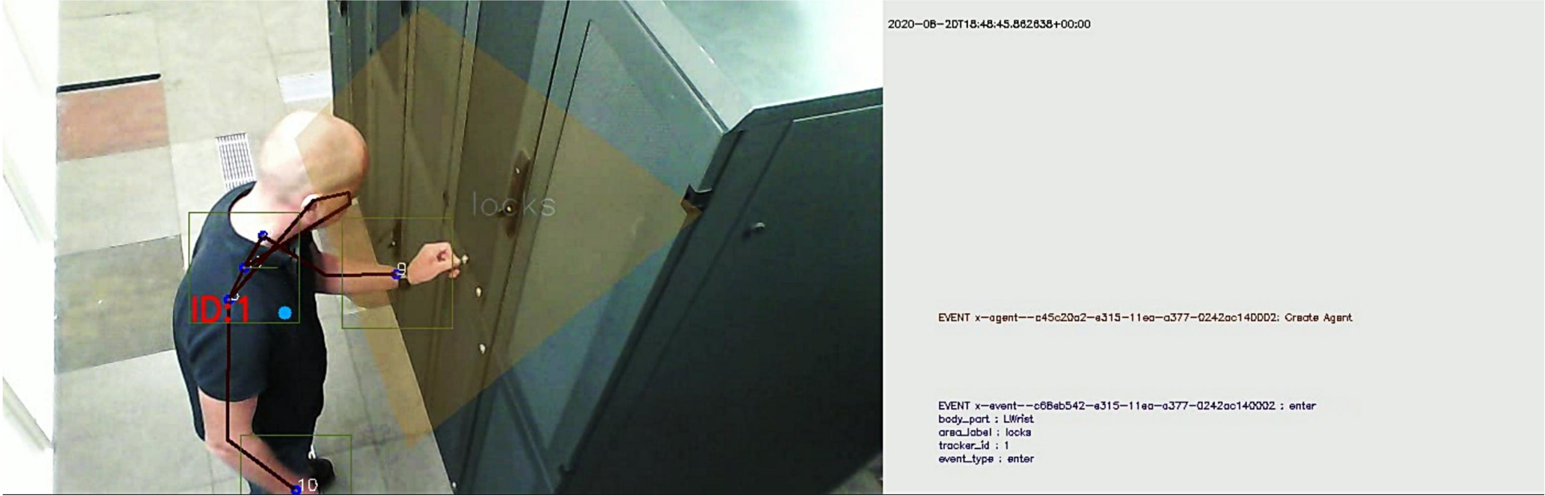
**Objective:** Detect and track interaction with rack's keyholes by two independent agents
